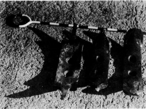
Figure 16. Cutters developed and used for cleaning transverse joints.
