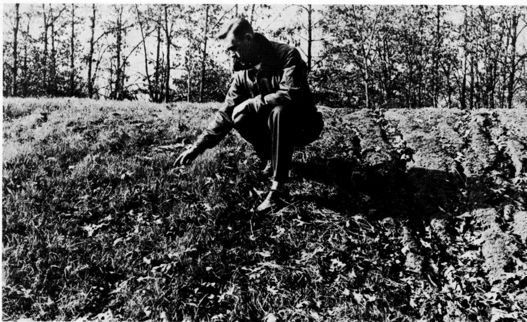
Figure 9. A CRD-189 surface-treated slope (at left) and an untreated control slope are studied several months after being established.
