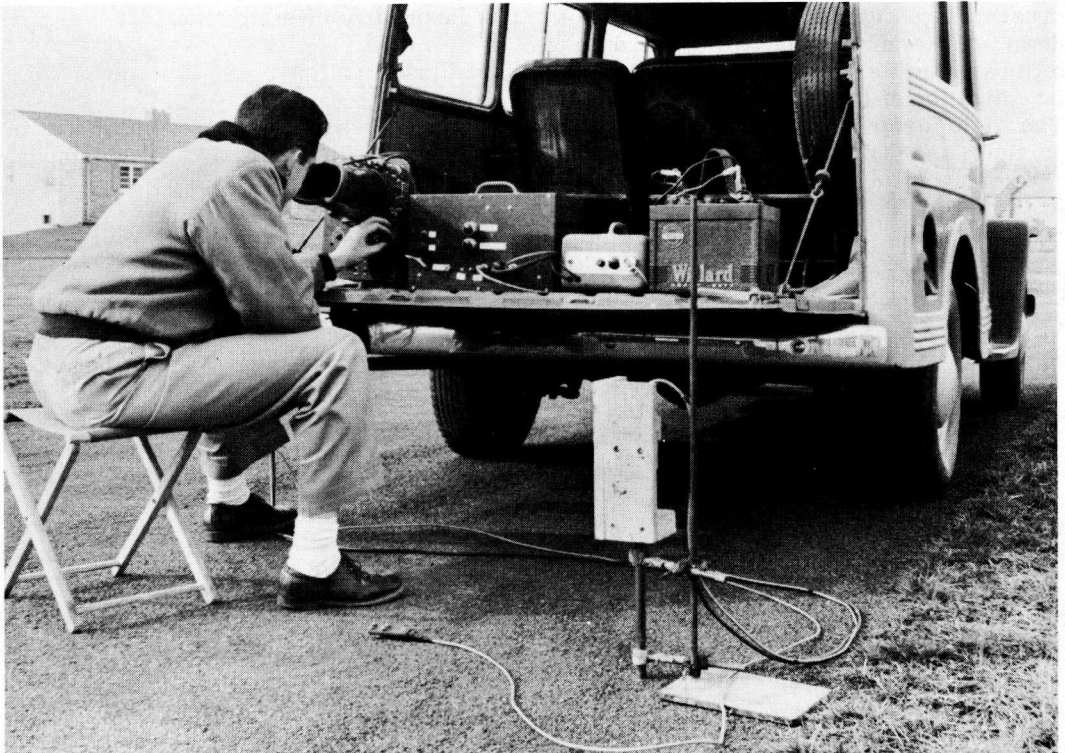
Figure 2. Measuring pulse velocity with portable field unit.
