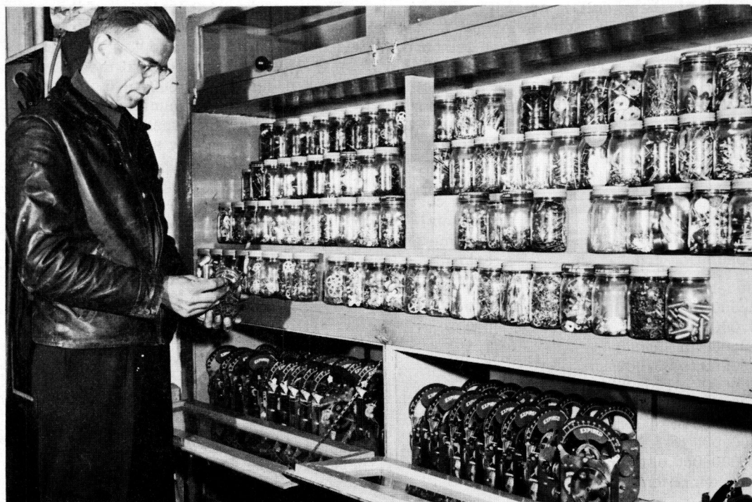
Figure 32. Parking meter parts are kept in glass containers in a systematic way in the repair shops of the Operations Section, Electrical Division, of the Highway Department of the District of Columbia. The meter mechanisms on the lower shelves have been fully repaired and are awaiting installation as the need arises.
