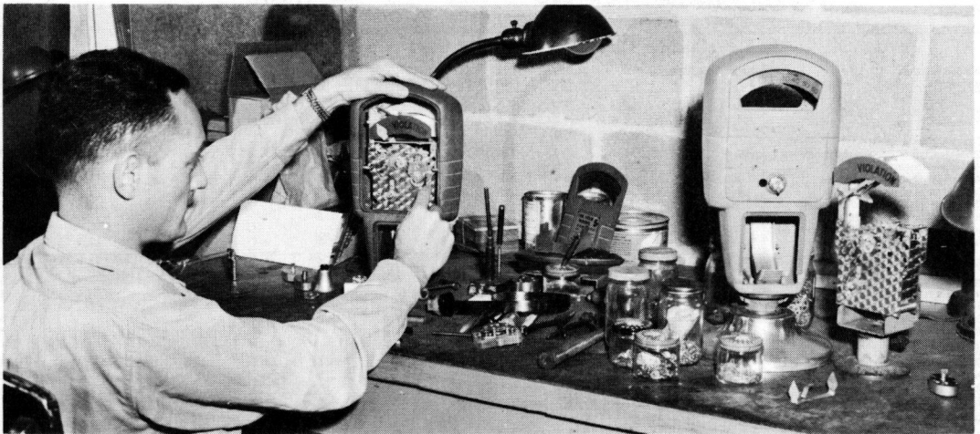
Figure 31. Sometimes minor adjustments of the parking meter mechanism will put it back into smooth operation.
