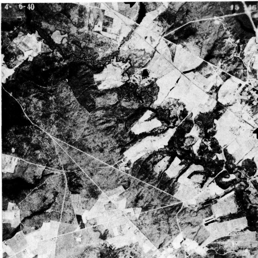
Figure 11. V-shaped gully development in an outlier. Severely dissected outlier parallels a stream. This outlier consists of granular material.
