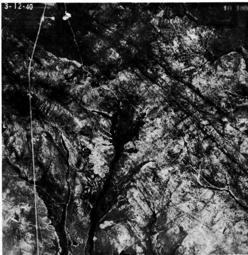
Figure 16. Long radial lines. The dark streaks prominent throughout, especially noticeable in upper-right corner. Lines continue irrespective of existing topography and alluvial channels.
