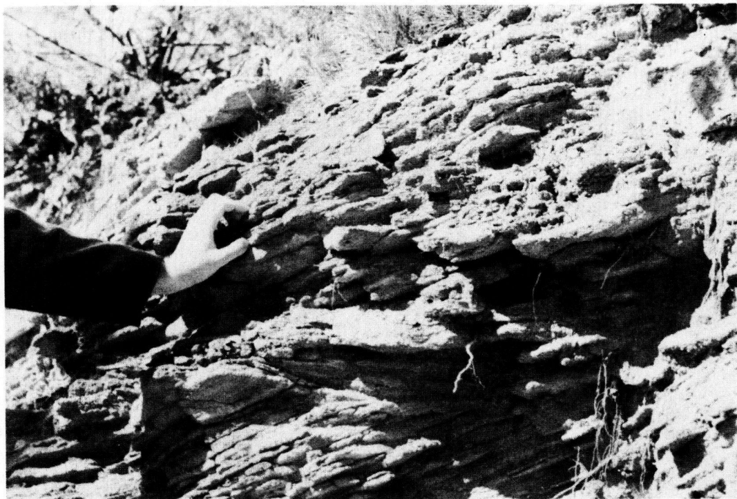
Figure 8. Iron-cemented sand and gravel. Bedded cementation has been encountered at depth in excess of 10 ft.
