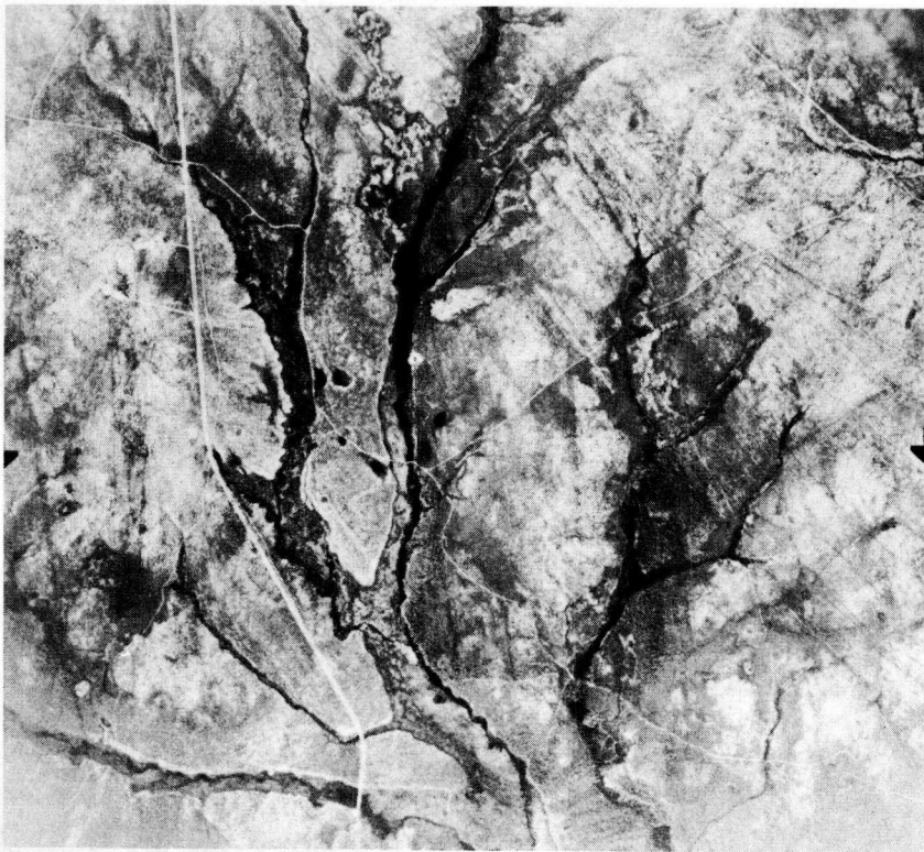
Figure 10. Typical amputated drainage pattern. Clearly defined edges of streams, with stubby appearance of minor tributaries. In upper left-hand corner, noticeable lack of any surface runoff pattern.
