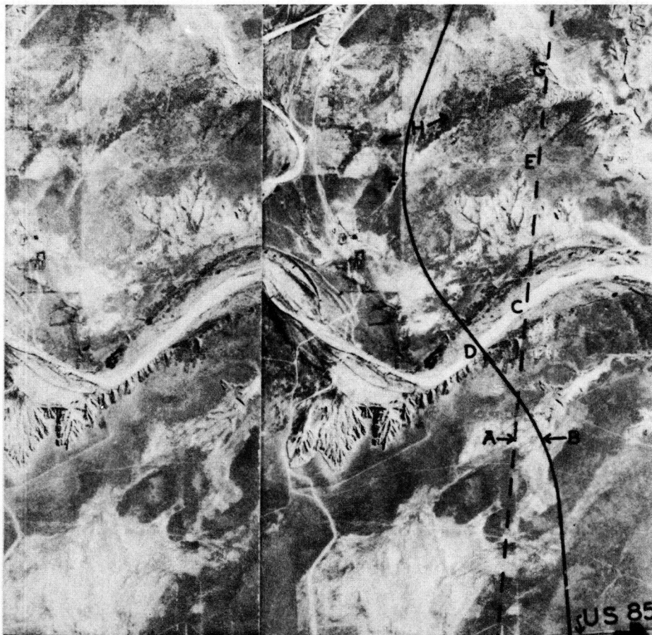
Figure 4. Airphotos on highway location. A stereopair in Niobrara County showing original alignment (A) at one end of a secondary location and the revised line (B). The revised line was developed by the engineer after securing airphotos for drainage area determination and deciding that the alignment could meet lower standards. The three-span, continuous, R.C. girder bridge required at D was at least one span shorter than required at C. Going through the saddle at F eliminated the adverse grades and deep cut that the hill at E would have necessitated. Alignment on the drainage division at H eliminated two drainage pipes required at G. This is in the Brule formation, Upper White River. (Courtesy of Jack Ammann, photogrammetric engineer.)
