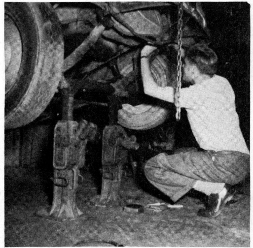
Figure 13. Marking frame to determine permanent deformation of different sections.
