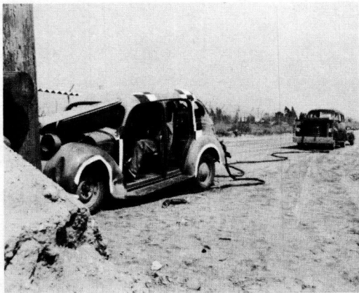
Figure 3. 1½-ton carryall used to push test car into barrier.
