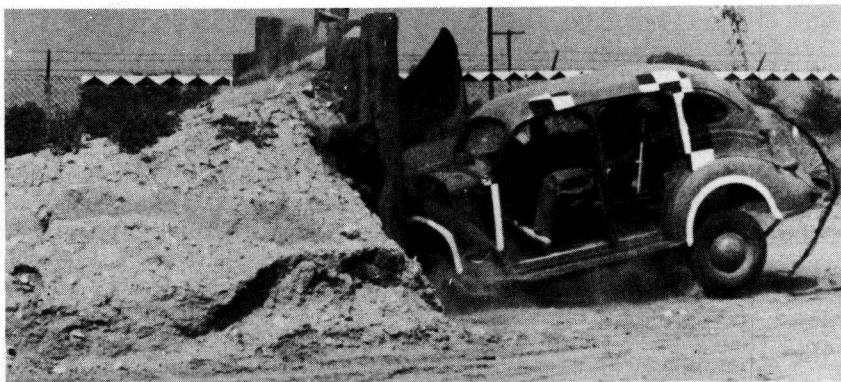
Figure 6. Checker board pattern on car for calibration with photographic film.
