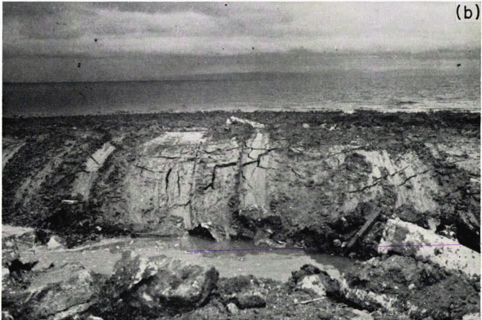
Figure 5. Type of mud wave produced by failures: (a) shear-type failure; (b) squeeze-type failure.
