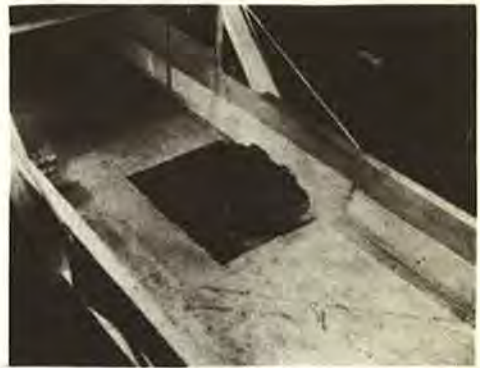
Figure 11. City Inlet, Series H, \sqrt{s/n} = 14.0 , Q_G = 1.00 , Q_I = 0.77 , Q_C = 0.23 cu ft per sec.
