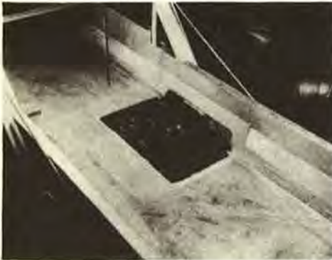
Figure 10. Highway Department Inlet, Series G, \sqrt{s/n} = 14.0 , Q_G = 1.00 , Q_I = 0.81 , Q_C = 0.19 cu ft per sec
