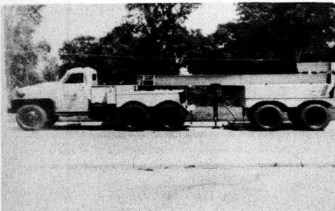
Figure 1. Truck-Trailer Unit Used for Plate Bearing Test Reaction - Ohio
