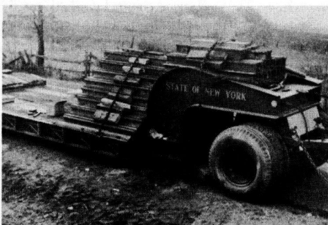
Figure 8. View of Loading Equipment Used in Fall of 1948 - Showing Loaded 30-Ton Trailer - Jacking equipment set in rear of goose-neck behind wheels. State of New York
