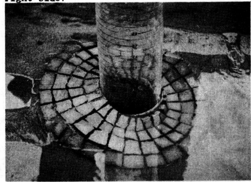
Loose-jointed block mat B1g at end of test. ←
