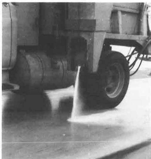
Figure 6. Dribbler applying evaporated salt.
