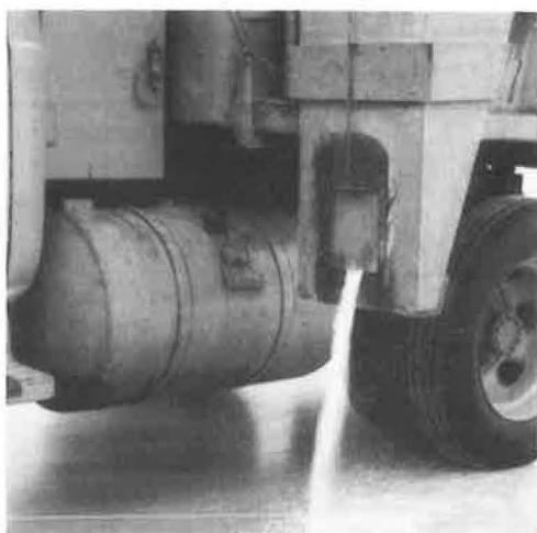
Figure 7. Dribbler applying calcium chloride and sodium chloride mixture.
