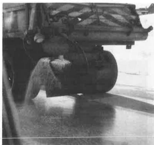
Figure 8. Disc spinner applying abrasive mixture.
