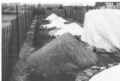
Figure 24. Test site for outdoor storage of chloride salt.
