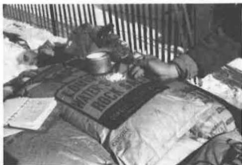
Figure 26. Method of taking moisture sample from packaged NaCl.
