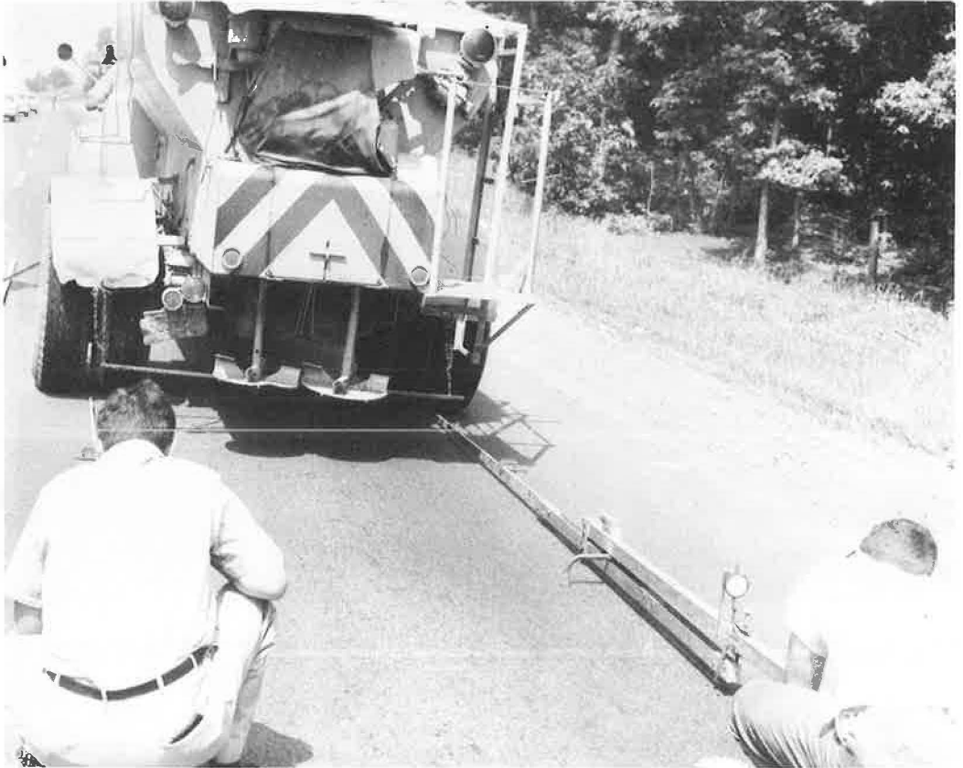
Figure 2. Truck moving ahead and stopping with load wheels several feet ahead of point of measurement.
