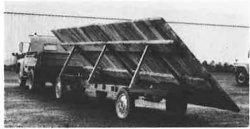
Figure 6. Test trailer used as portable steep shoulder and ditch section (deck = 1\frac{1}{4} :1 slope).
