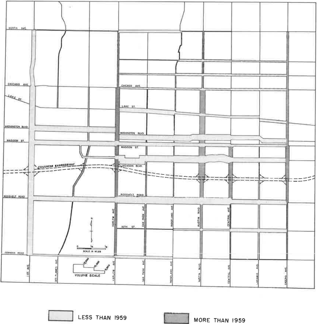
Figure 2. Redistribution of traffic volume on average weekday on arterial streets due to opening of Congress Expressway.
