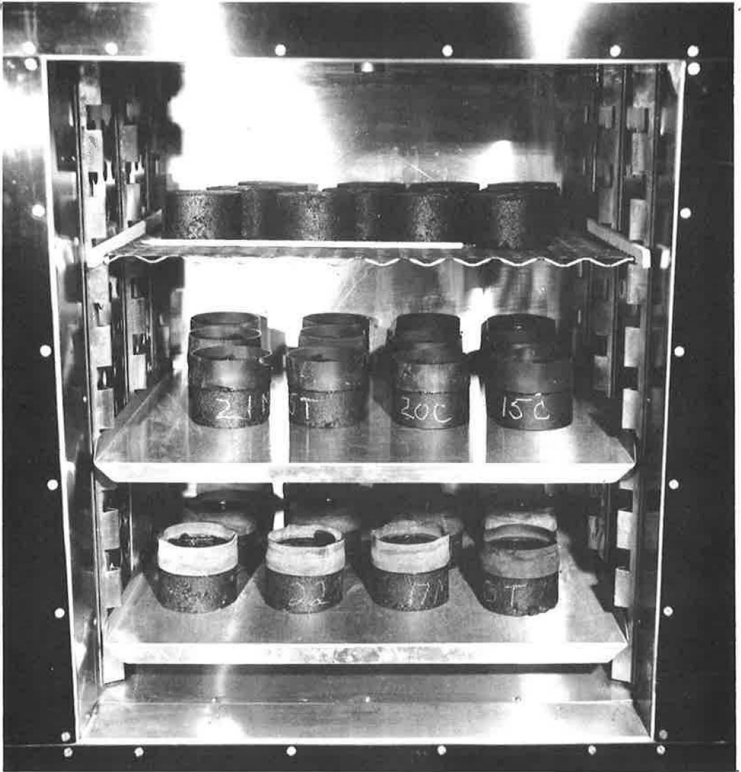
Figure 1. Test specimens in test cabinet.
