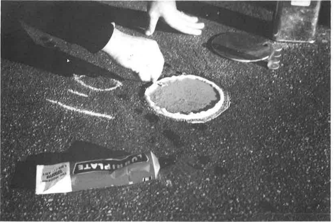
Figure 23. "Grease ring" permeability test.
