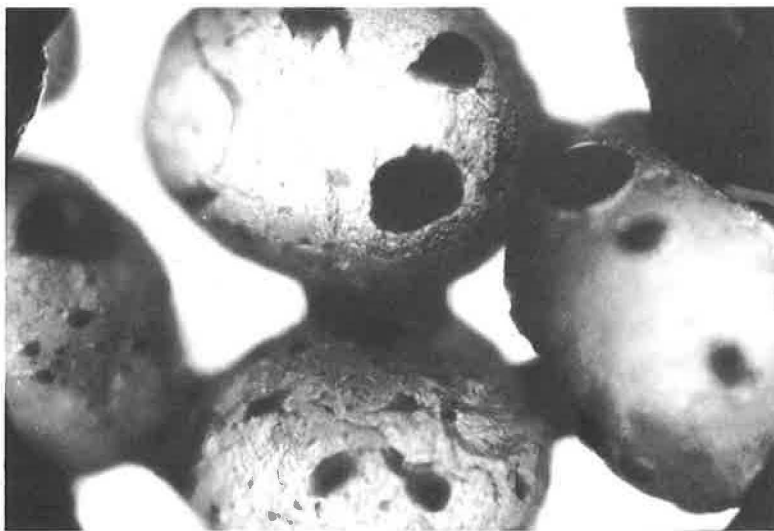
Figure 16. Photomicrograph before stripping test of untreated sand-asphalt mix (see Fig. 15a).
