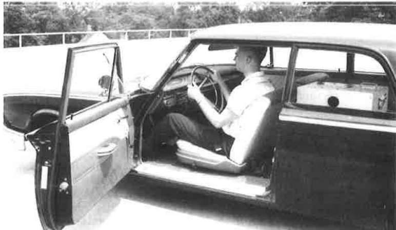
Figure 1. Test car with drivometer mounted on rear seat.
