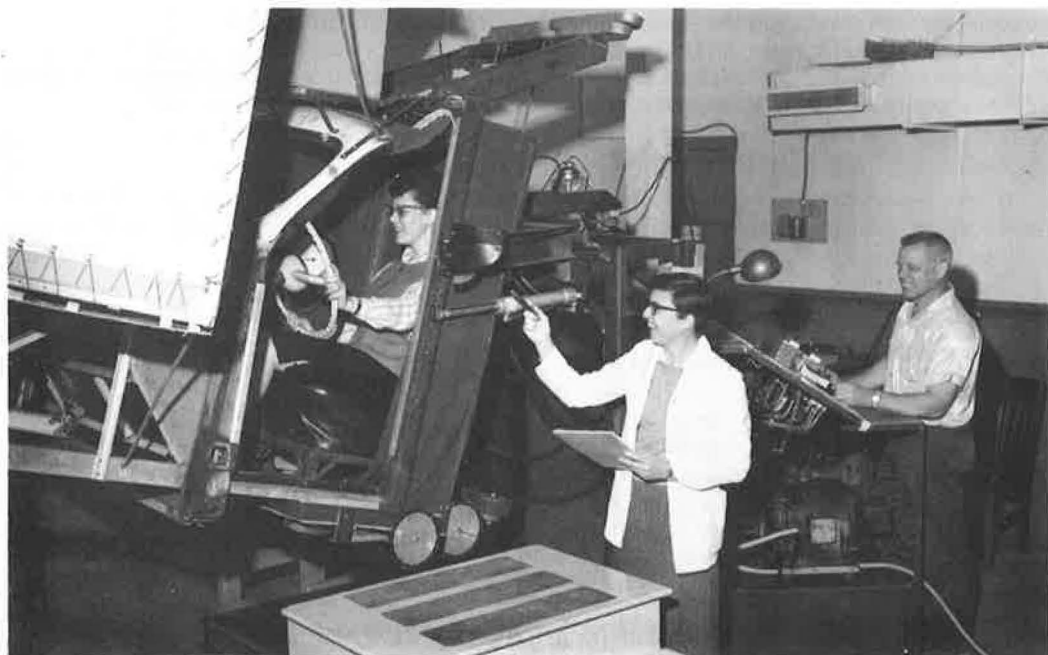
Figure 2. Driver demonstrating one position of the moving-base device.
