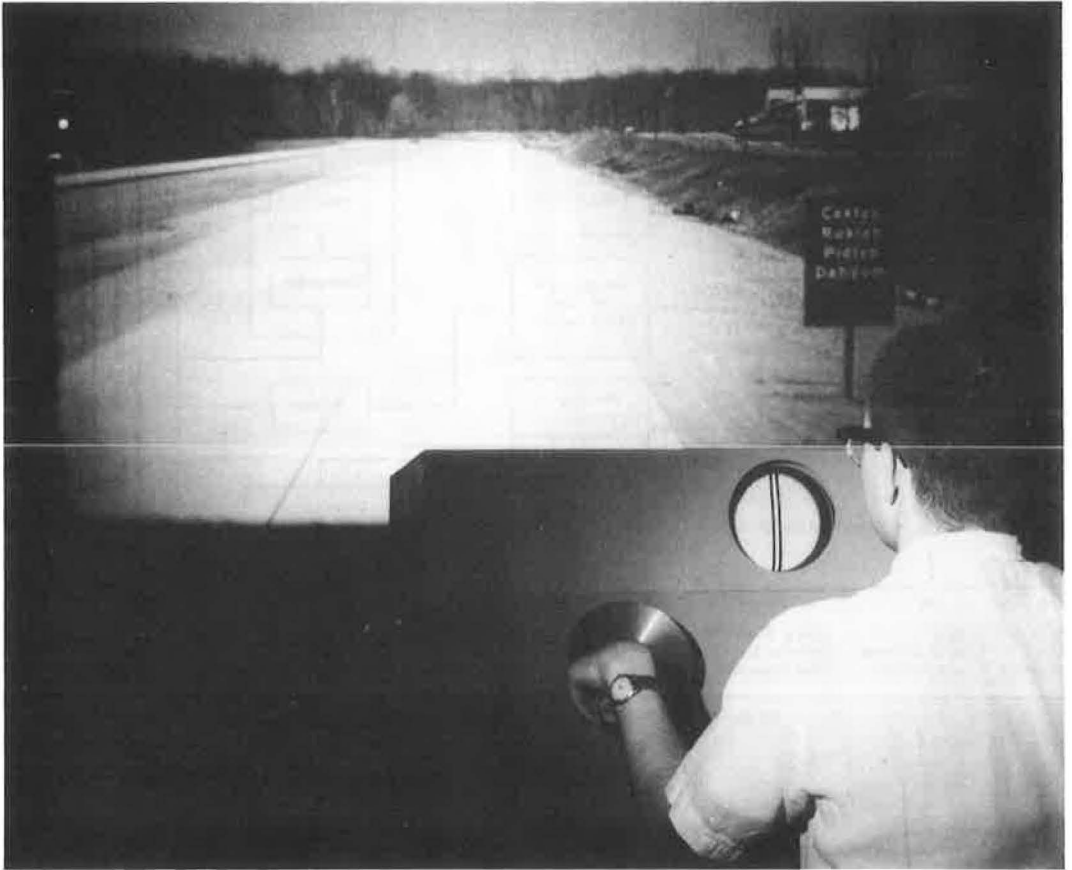
Figure 5. Subject seated at driving console performing tracking and search-and-recognition tasks.
