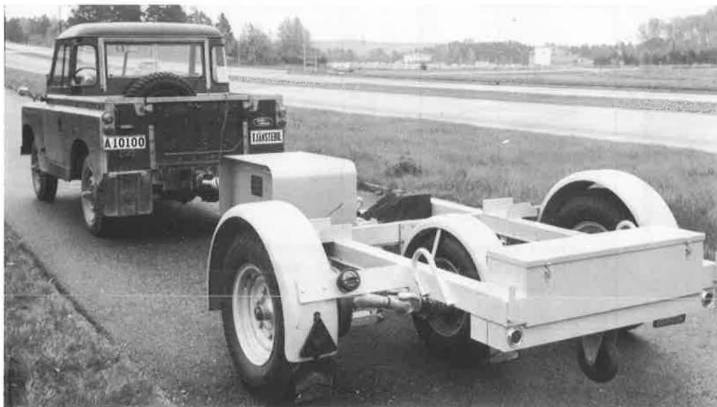
Figure 27. Swedish 3-wheel trailer and runway and road skid resistance test vehicle (Skiddometer).
