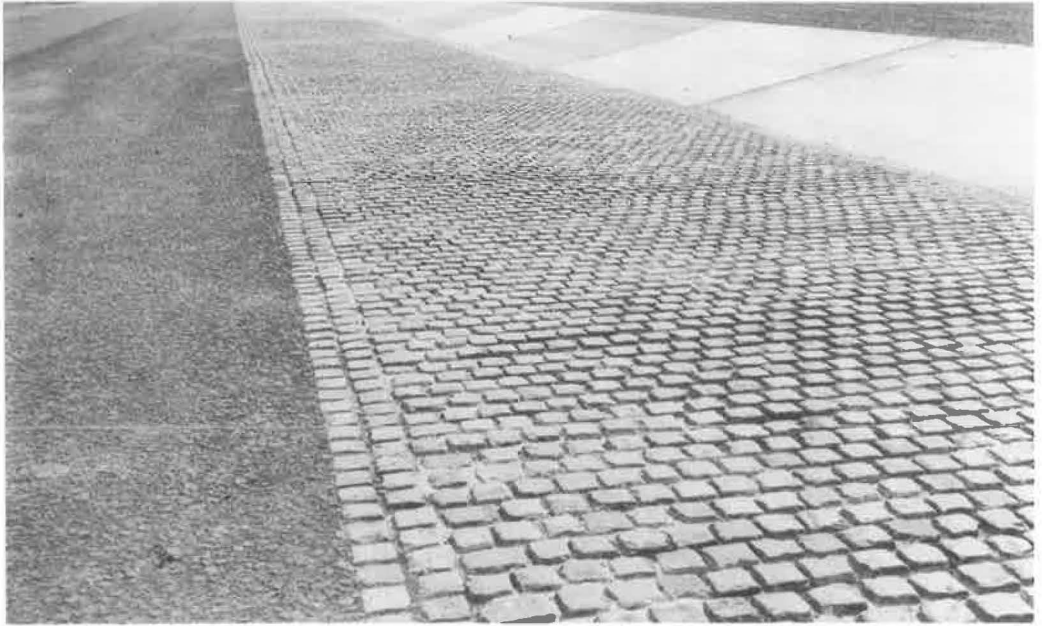
Figure 19. Test sections, Dunlop Proving Ground—tar macadam, granite setts, and portland cement concrete.
