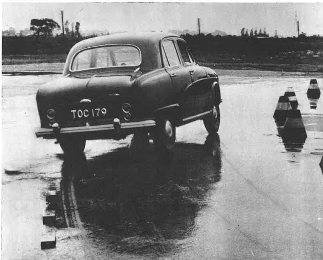
Figure 18. Dunlop cornering test to establish maximum breakaway speed on a marked 100-ft radius curve.
