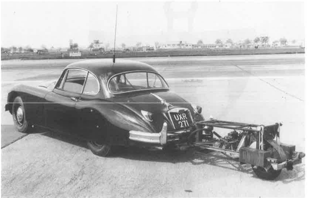
Figure 16. British car and trailer for braking-force skid resistance measurements at speeds up to 100 mph.
