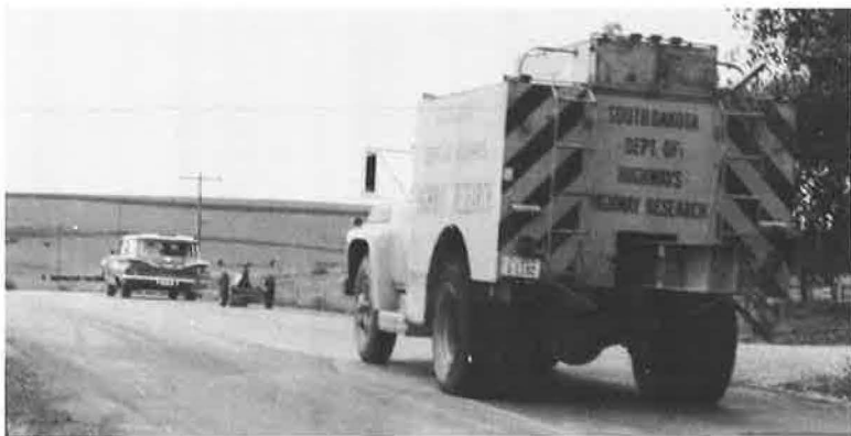
Figure 4. CHLOE profilometer in operation, followed by warning truck.
