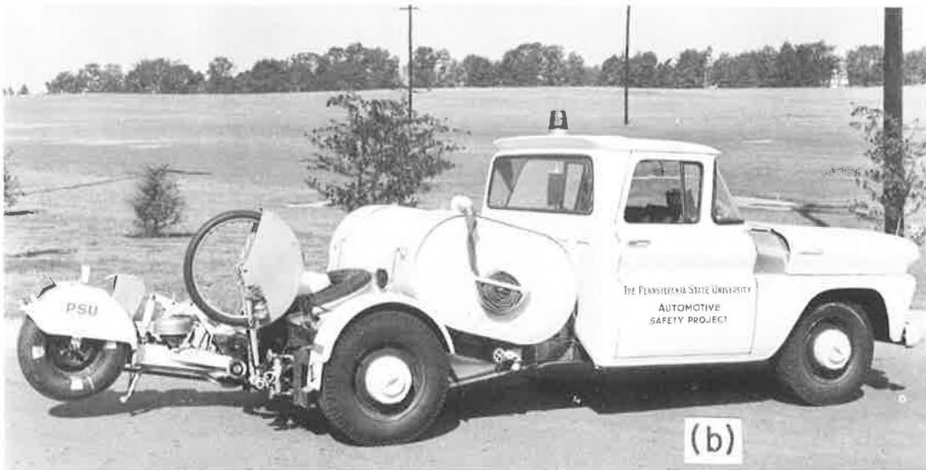
Figure 7. Penn State road friction tester: (a) trailer in test position; and (b) trailer in transport position.
