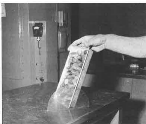
Figure 2. Outer stones stable at \alpha = 70^\circ + .
