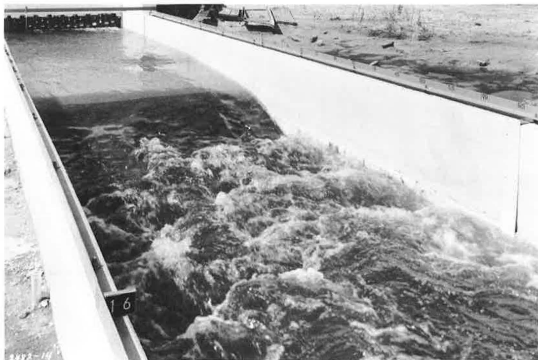
Figure 5. Flow through model, 20 cfs.
