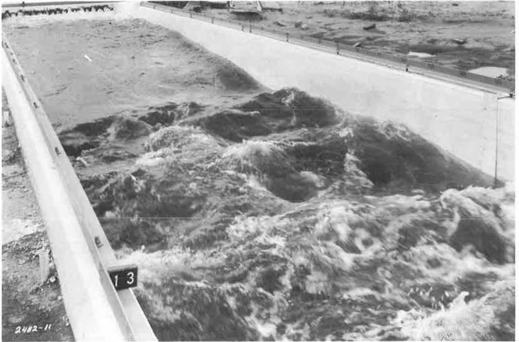
Figure 6. Flow through model, 60 cfs.
