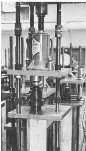
Figure 9. Hydraulic jack used in spring-loading system.
