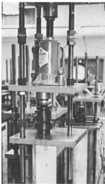
Figure 9. Hydraulic jack used in spring-loading system.
