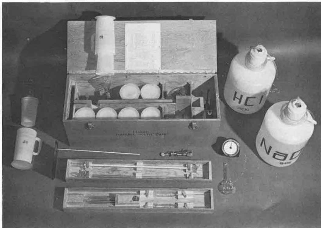
Figure 19. Field kit for titration test.
