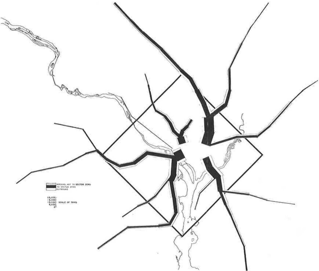
Figure 10. Transit traffic flow for NCTA recommended system.
