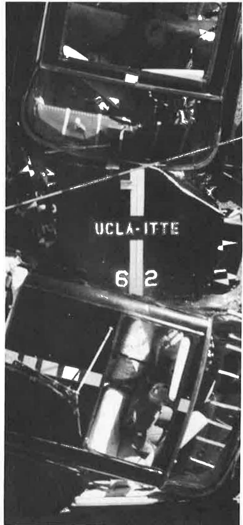
Figure 12. Impact forcing door open.
