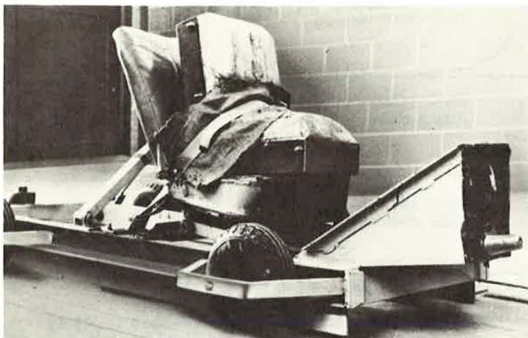
Figure 2. Swedish dynamic test cart, with lead cone fixed on front end—rigid dummy shown in bucket seat, held by lap belt.
