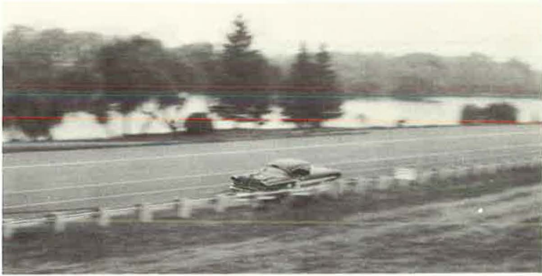
Figure 25. Successful 65-mph guardrail test.
