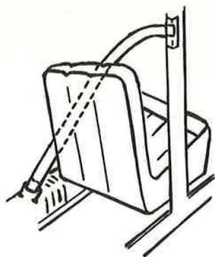
Diagonal belt fitted to door pillar.
