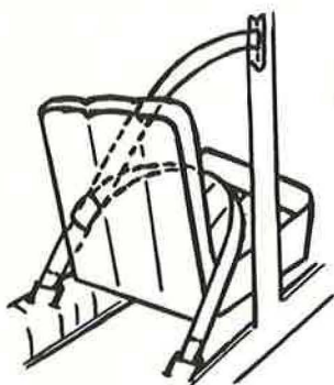
Combined lap belt and single diagonal shoulder strap. (Alternatively, shoulder strap may be brought over back of seat and anchored to floor instead of door pillar.)
