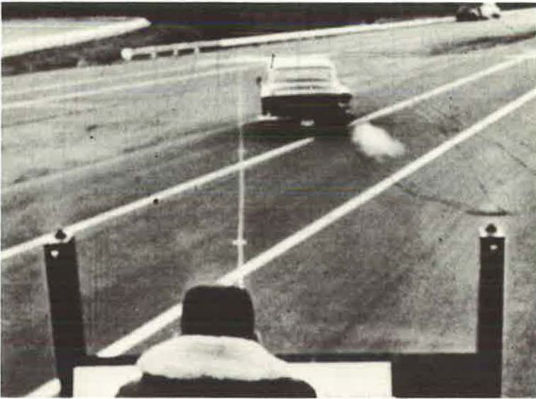
Figure 22. 35-mph guardrail test showing remote control.
