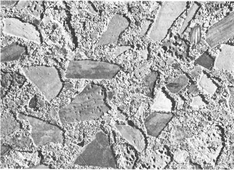
Figure 22. KC-11, sawed surface, \times 1\frac{1}{2} , etched with 3N hydrochloric acid. Acid made a smooth, even etch on most particles. Pocked appearance of some particles is due to dissolved-out fossils. All coarse aggregate particles are in negative relief.
