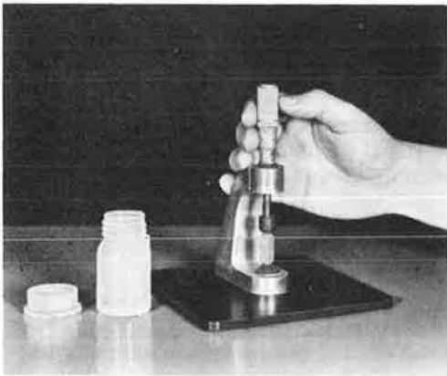
Figure 9. Simple test for measuring rock samples for expansion in alkali solution.
