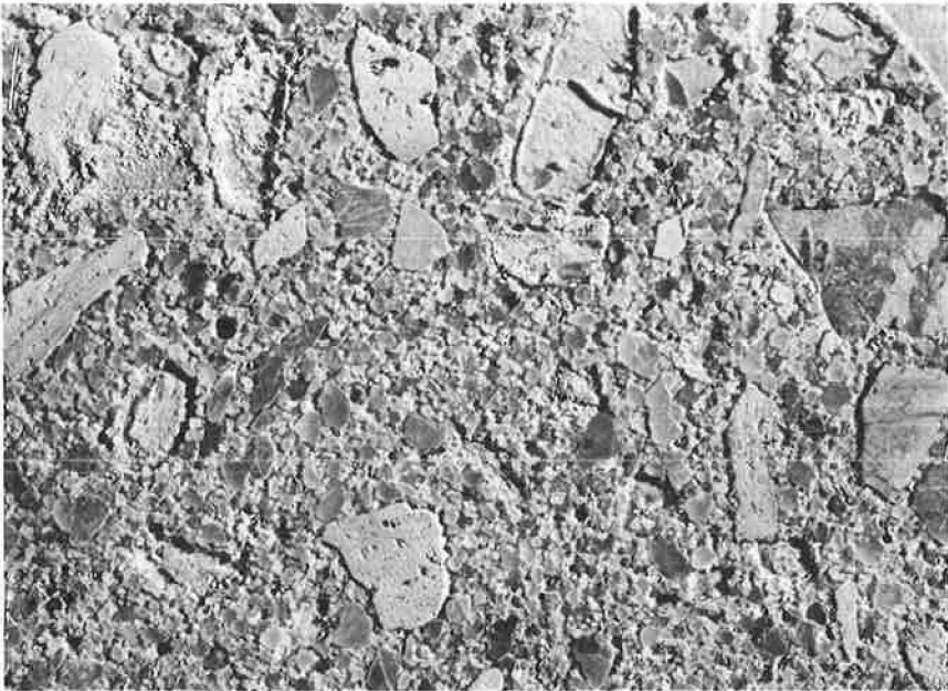
Figure 15. KC-7, sawed surface, \times 1\frac{1}{2} , etched with 3N hydrochloric acid. Rims that were present in mortar surrounding cherty particles were destroyed by the acid etch. Rims are present in two limestone particles in upper part of photograph.
