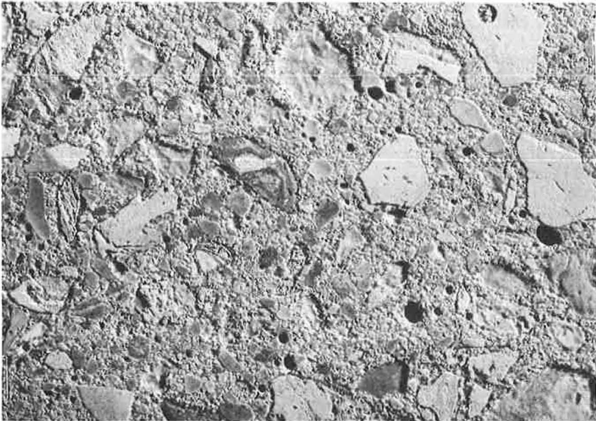
Figure 13. KC-6, sawed surface, \times 1\frac{1}{2} , etched with 3N hydrochloric acid. Light colored, spongy-textured, cherty particles were more resistant to acid attack and are therefore in relief above etched concrete surface. Limestone particles, being less resistant, are in negative relief.
