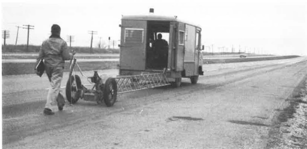
Figure 1. CHLOE profilometer in use. Man behind profilometer records cracking, patching and rut depth, to be used with CHLOE and texturemeter data in calculating serviceability index. Profilometer is loaded in towing vehicle for travel between test sections.
