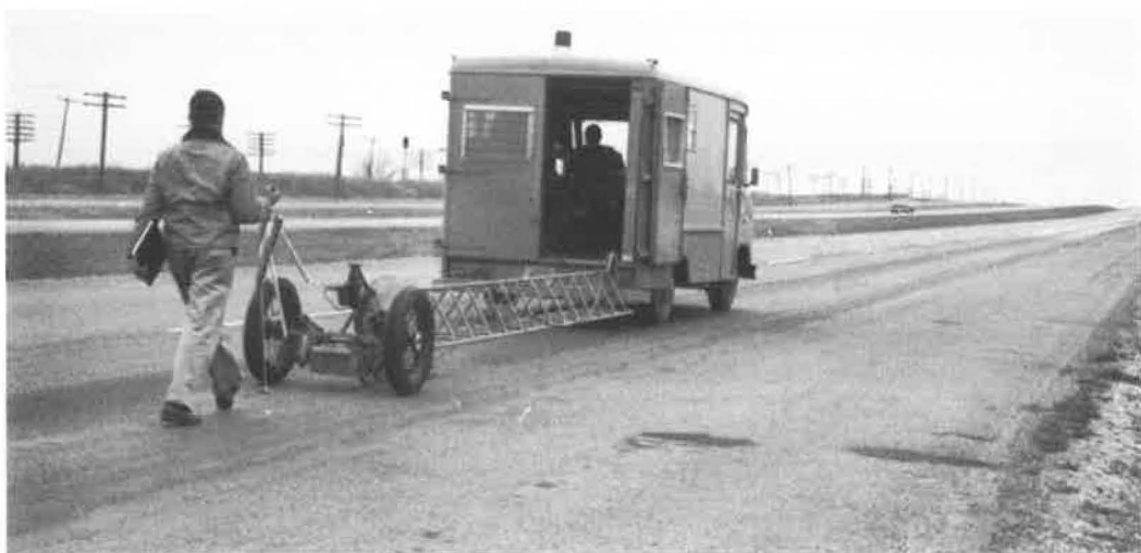
Figure 1. CHLOE profilometer in use. Man behind profilometer records cracking, patching and rut depth, to be used with CHLOE and texturemeter data in calculating serviceability index. Profilometer is loaded in towing vehicle for travel between test sections.
