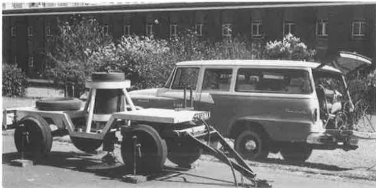
Figure 1. Station wagon and trailer set up for an impedance test.
