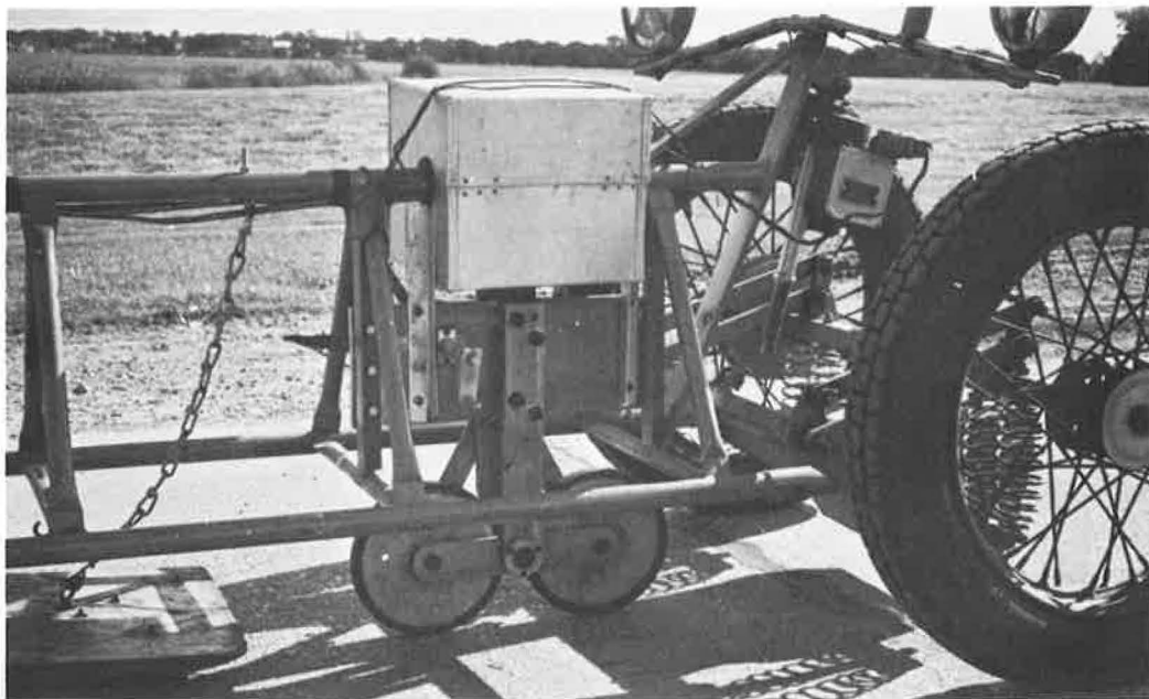
Figure 2. Close-up of slope wheels of CHLOE profilometer. Device measures angle between trailer tongue and link between slope wheels.
