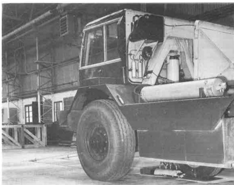
Figure 9. Heavy wheel load skidding machine showing test wheel mounted on calibration rig.
