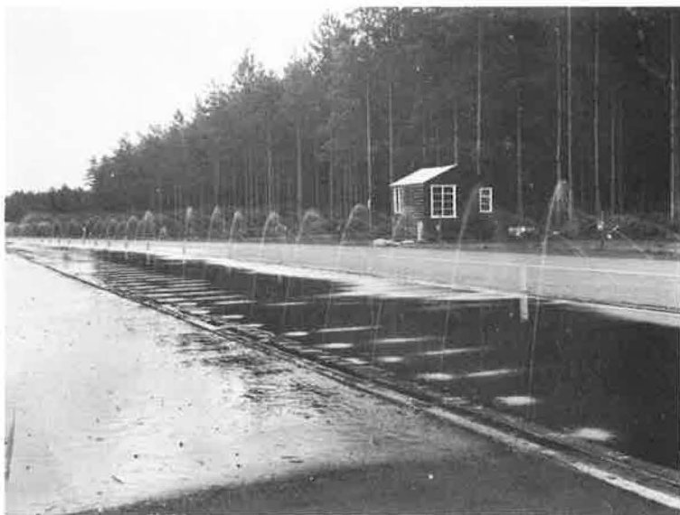
Figure 4. Crowthorne Research Track spraying system in operation under comparatively low pressure.
