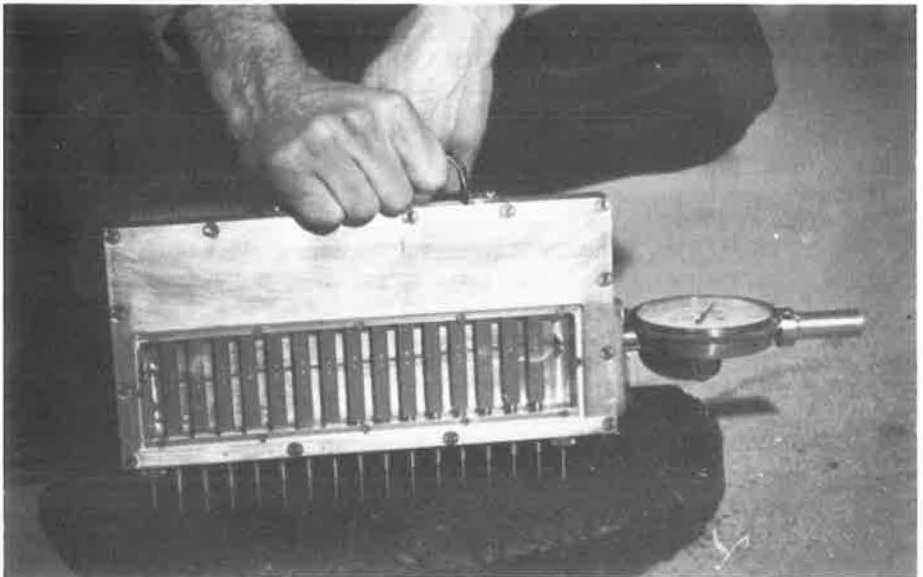
Figure 4. Texturemeter applied to laboratory specimen of asphaltic concrete. Road surfaces give dial readings ranging from 0 to about 0.100 in.
