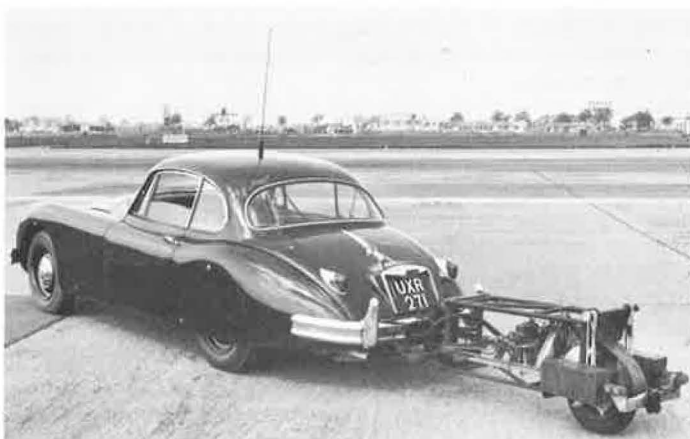
Figure 5. Test trailer used for measurement of braking force coefficient.
