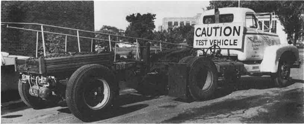
Figure 5. Tire dolly test rig.
