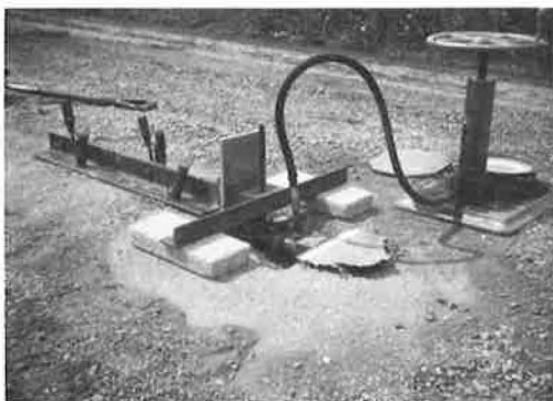
Figure 2. Typical failure of soil-aggregate surface course in Burggraf shear test.
