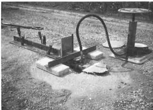
Figure 2. Typical failure of soil-aggregate surface course in Burggraf shear test.
