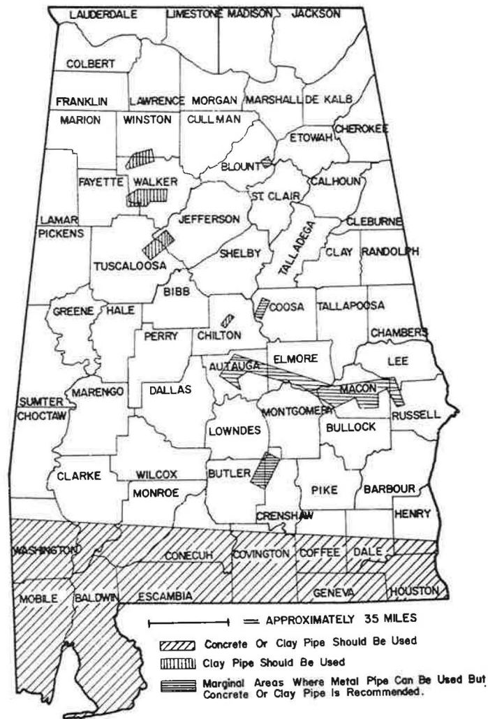
Figure 4. Pipe zoning map of Alabama showing areas where specific types of drainage pipe are recommended to provide longer performance life.
