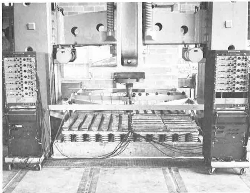
Figure 4. Load test on concrete slab.
