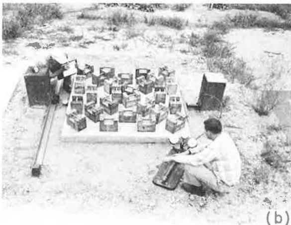
Figure 1. (a) Slabs between abutments, and (b) 5-in. slab loaded to weight equivalent of 11-in. slab.
