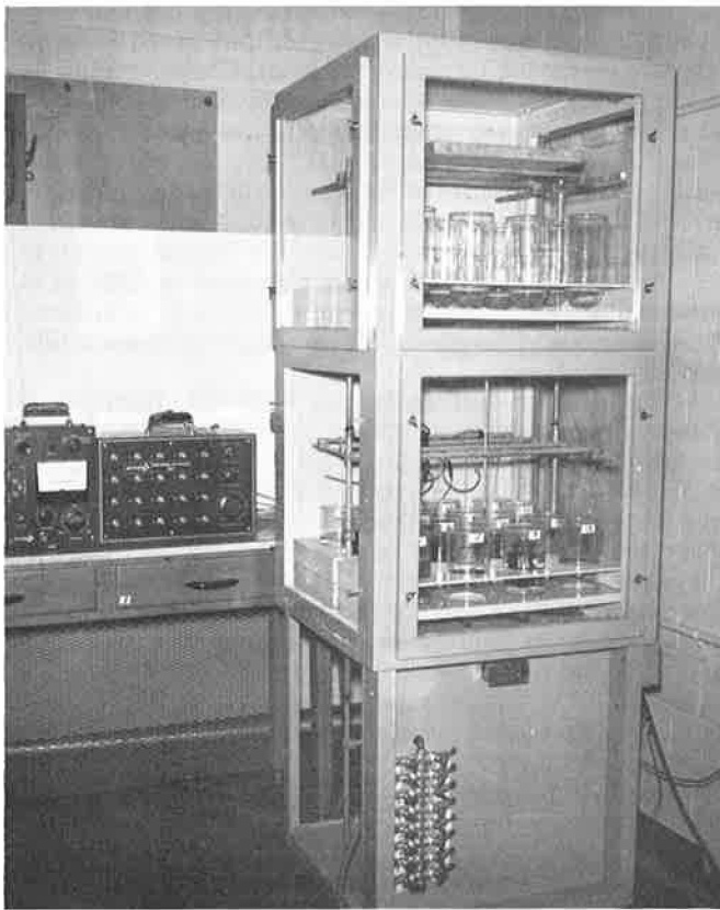
Figure 6. Apparatus for alternate immersion of specimen in ice melting solutions and suspending in air.
