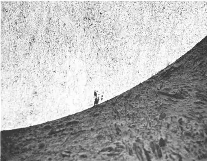
Figure 10. Photomicrograph of cross-section of specimen 13A after cyclic exposure under stress to NaCl solution for 238 hr (60X)—HF etch.
