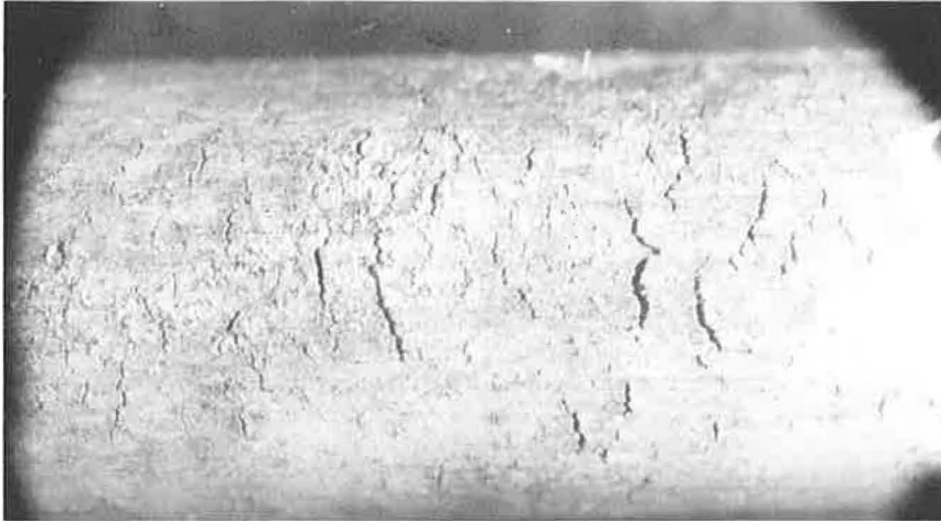
Figure 2. Specimen corroded by exposure to NaCl solution and pulled.
