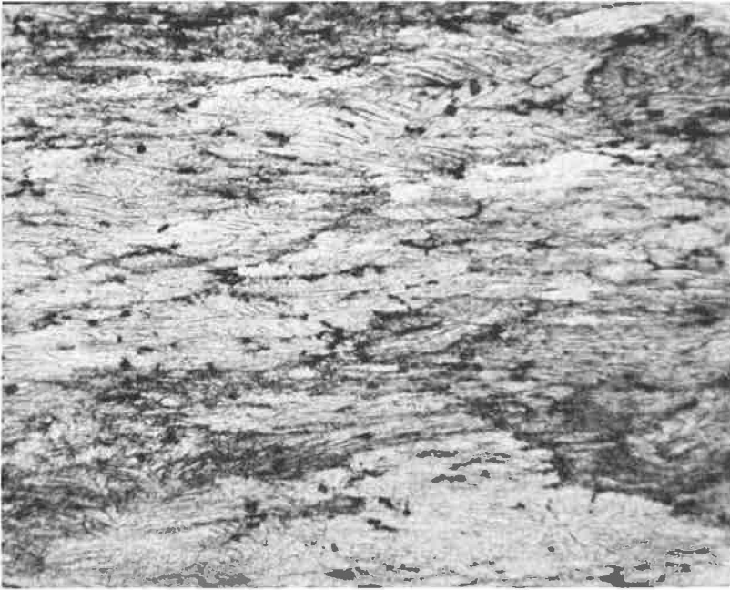
Figure 7. Photomicrograph of typical structure (parallel to long axis) of forged 7079-T6 billet (60X)—Keller's etch.
