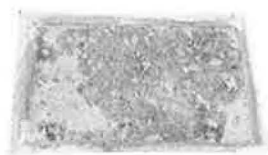
Figure 2. Effect of linseed oil surface treatments on scaling: 105 cycles, slump 6.0 in., air 1.4 percent.
