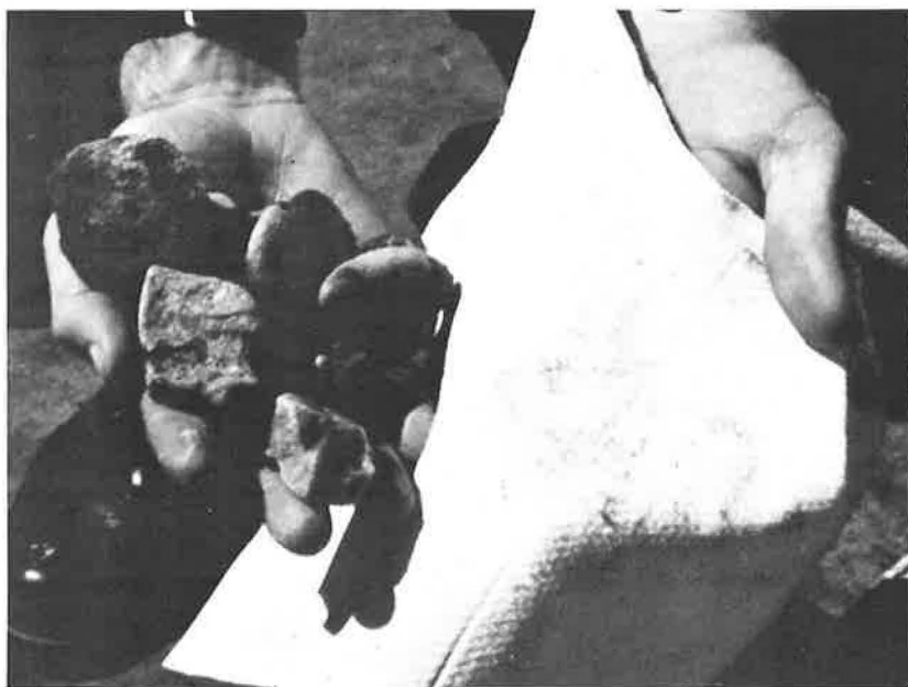
Figure 2. Degradation of 1\frac{1}{2} -by \frac{3}{4} -in. pcc aggregate.
