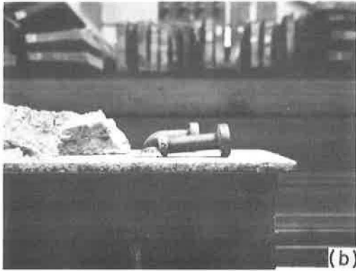
Figure 18. Stud fatigue failure adjacent to uncracked connector.
