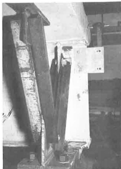
Figure 4. End braces and end slip measuring device.
