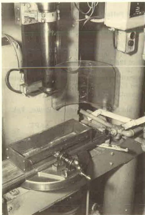
Figure 21. Mold and carriage which holds steel mold during compaction.
