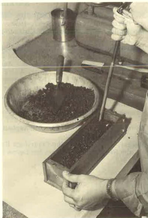
Figure 22. AC mix being rodded with \frac{3}{8} in. bullet-nosed rod.
