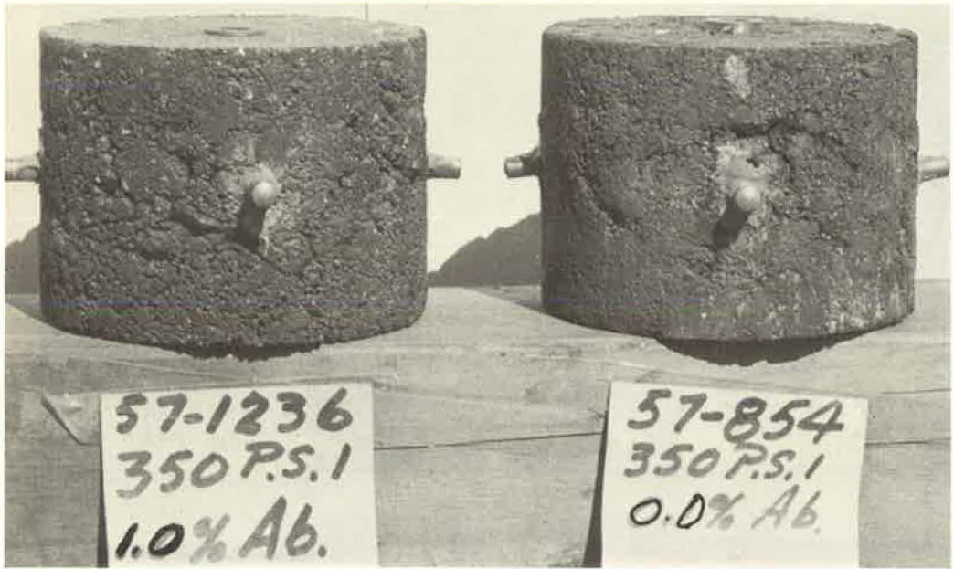
Figure 6. Stainless steel pins cemented to sides of specimen to measure volume changes.
