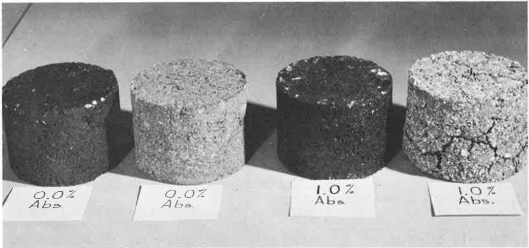
Figure 7. Absorptive and nonabsorptive AC briquettes; dark-colored specimens stored in cabinet for 6 yr, and light-colored specimens exposed on roof for 6 yr.
