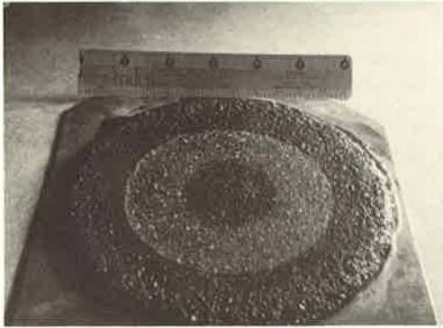
Figure 5. Slurry seal test specimen—excellent: A = < 1 percent, S = < 10 percent, T_R = 85-100 percent.
