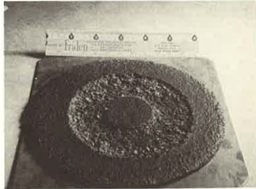
Figure 8. Slurry seal test specimen—unsatisfactory: A = > 10 percent, S = > 15 percent, T_R cannot be determined.
