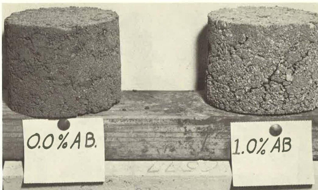
Figure 4. Nonencapsulated specimens exposed on roof 6 mo: left, nonabsorptive aggregate; right, absorptive aggregate.
