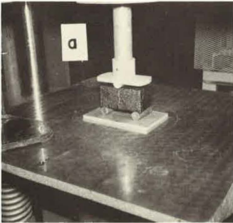
Figure 5. Specimens in position for test: (a) flexure, and (b) triaxial compression.
