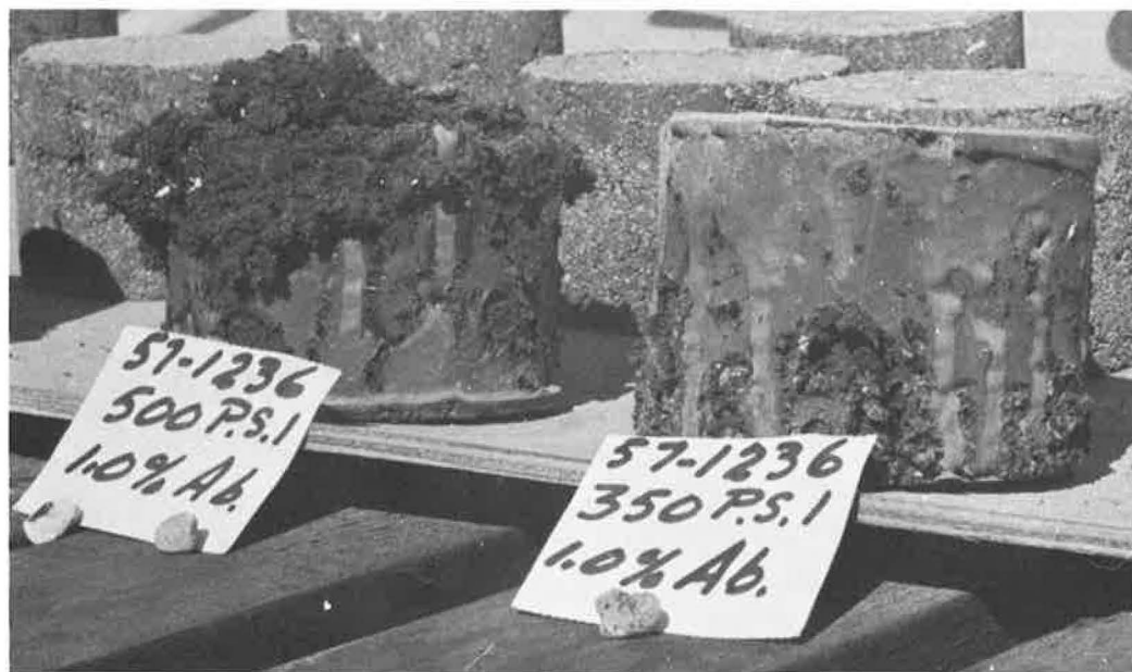
Figure 1. Epoxy-coated specimens, made from absorptive aggregates, exposed on roof 6 mo: left, specimen compacted at 500 psi; right, specimen compacted at 350 psi.
