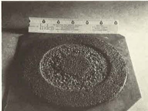
Figure 7. Slurry seal test specimen—fair: A = 5-10 percent, S = 10-15 percent, T_R = 65-80 percent.
