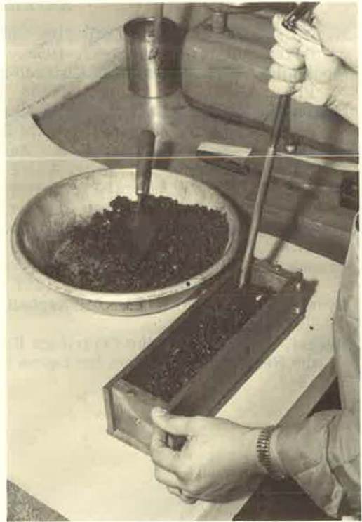
Figure 22. AC mix being rodded with \frac{3}{8} in. bullet-nosed rod.
