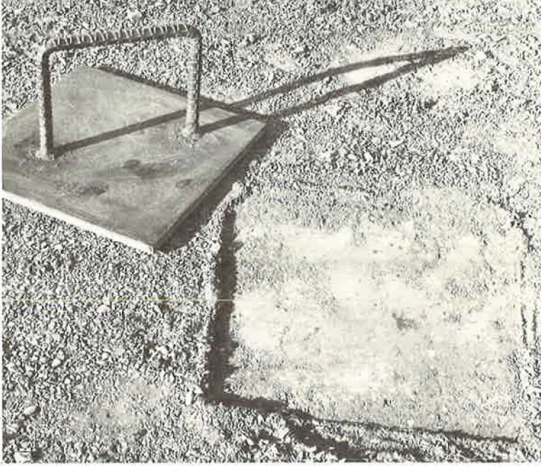
Figure 17. Steel plate, \frac{1}{2} by 12 by 12 in., with welded reinforcing bar for handle.
