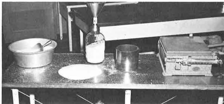
Figure 16. Sand-cone density apparatus being calibrated on 0.1-cu ft mold.
