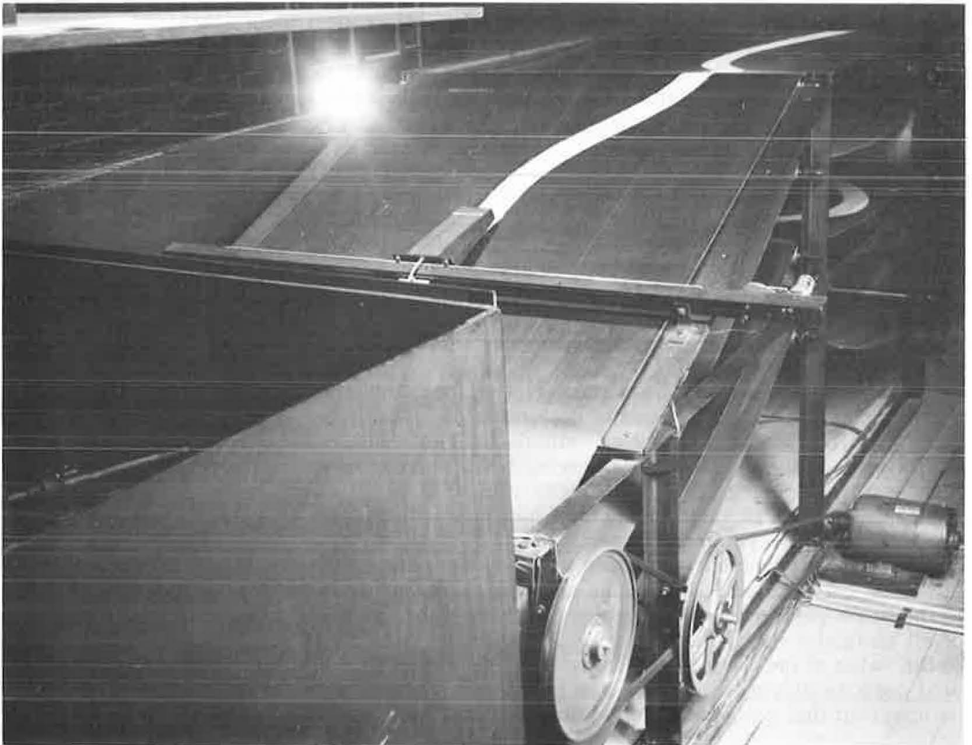
Figure 1. The roadway conveyor with the cursor above the simulated road; driver's cab is partly visible on the left, a glare light is on the glare conveyor.
