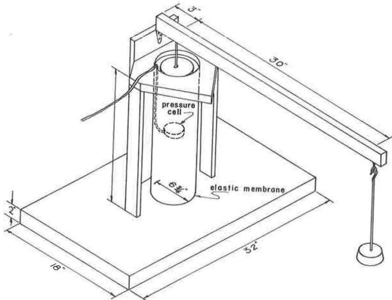
Figure 13. Calibration apparatus.
