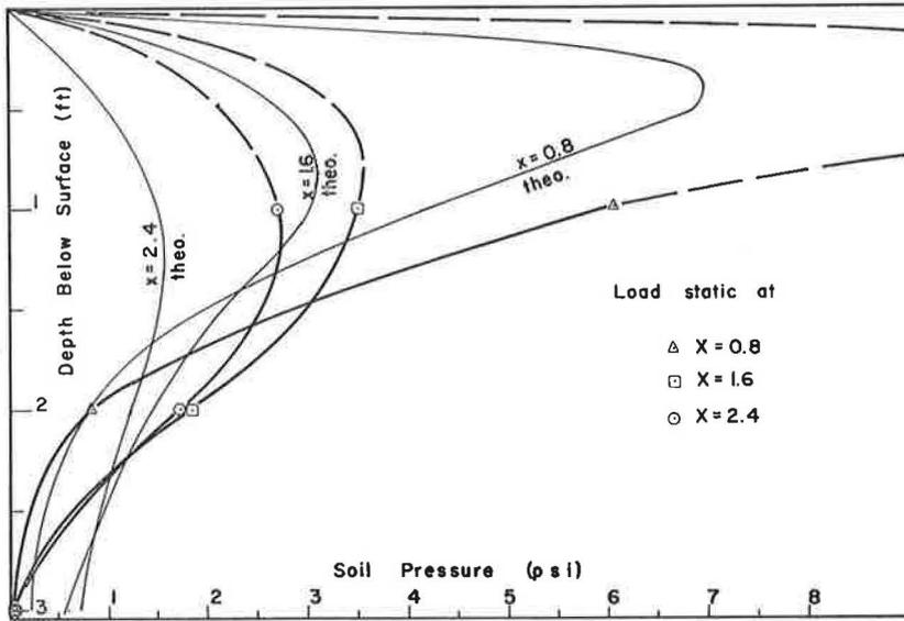
Figure 29. Soil pressure at rigid wall for different rear wheel locations (native).
