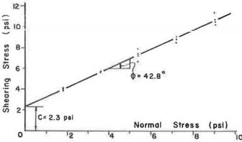
Figure 9. Direct shear envelope for native backfill material.
