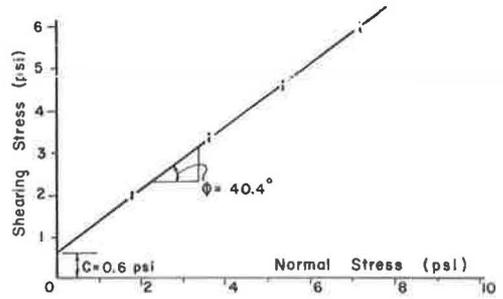
Figure 10. Direct shear envelope for sand backfill material.
