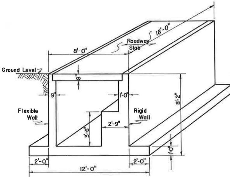
Figure 3. Test abutment.
