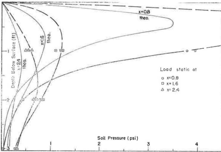
Figure 32. Soil pressure at flexible wall for different front wheel locations (sand).
