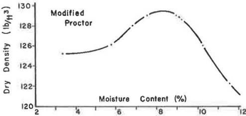
Figure 11. Moisture-density relationship for native backfill material.
