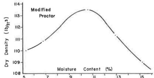
Figure 12. Moisture-density relationship for sand backfill material.
