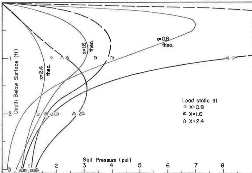
Figure 30. Soil pressure at rigid wall for different rear wheel locations (sand).
