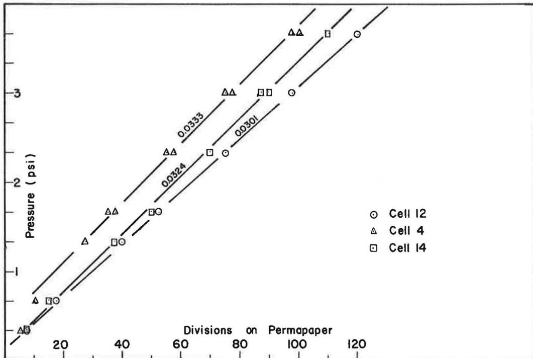
Figure 14. Calibration of can type pressure cells.
