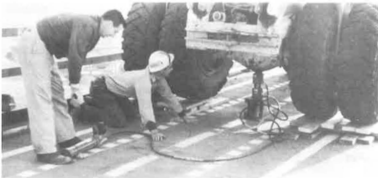
Figure 45. Cracking deck slab with 47-kip rear axle reaction on 10- by 14-in. plate to evaluate effects of slab cracking on load distribution.
