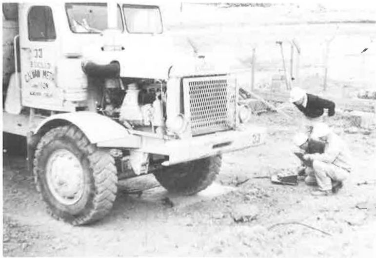
Figure 12. Typical measurement of test vehicle wheel reactions on Loadometer box.
