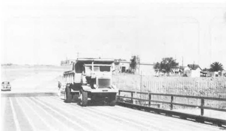
Figure 10. Test vehicle traversing prototype structure at crawl speed; painted striping on deck to facilitate transverse positioning.
