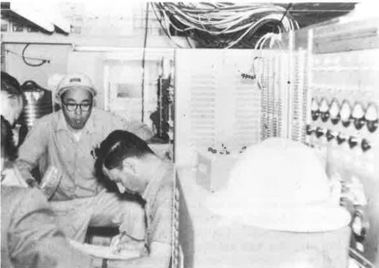
Figure 6. Interior view of instrumentation trailer with leads from 200 gages coming down through trailer ceiling.
