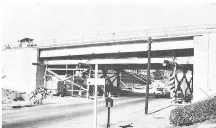
Figure 1. Overall view of prototype test structure, showing deflectometer scaffold, instrumentation trailer inclosure, and test vehicle.
