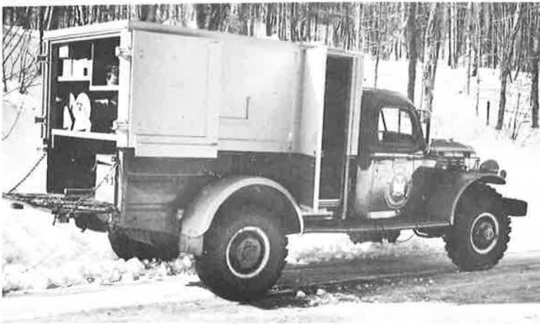
Figure 5. Seismic truck—door to instrument compartment is just forward of right rear fender.
