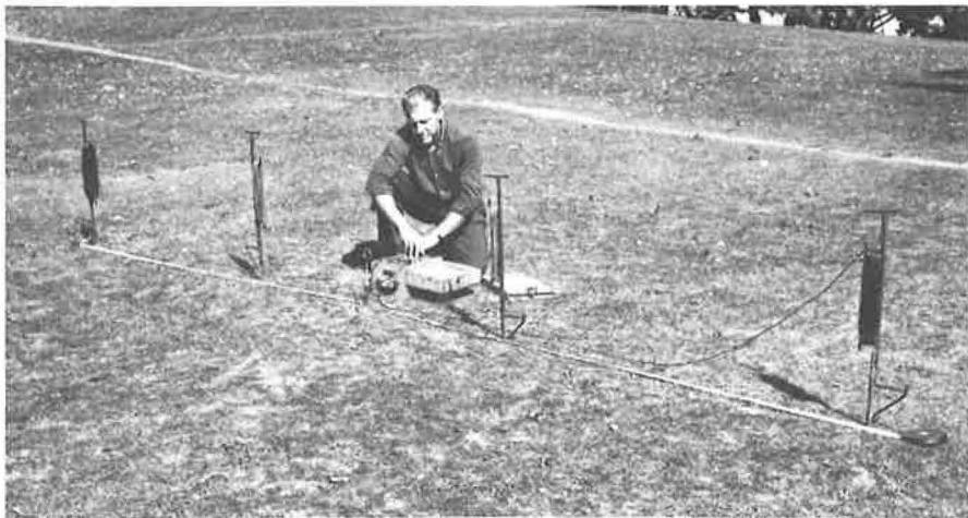
Figure 1. Resistivity instrument as set up to take readings.
