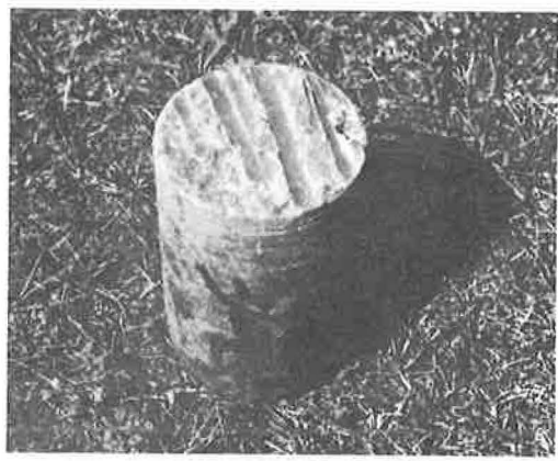
Figure 10. Core with top 3/4 in. broken off during drilling (note slick grooves made by spike drag), Iowa 37.
