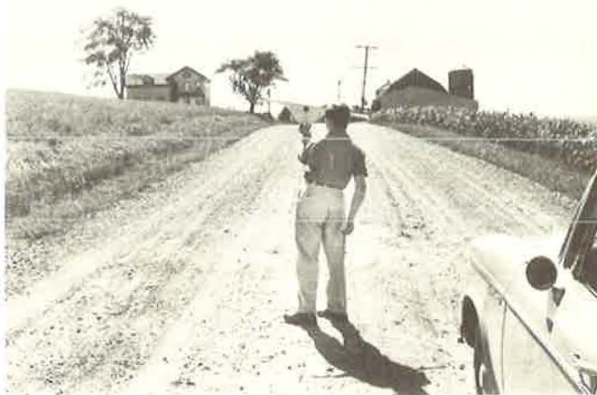
Figure 12. Measuring transverse terrain slope.
