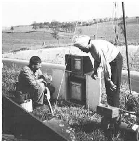
Figure 2. Microclimate equipment in operation along highway slope showing recorders used in measuring soil temperature and light intensity.
