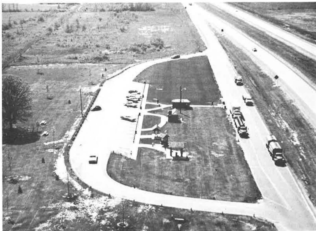
Figure 3. Aerial view of typical Michigan rest area, showing access ramp, parking areas, and distribution of user facilities.
