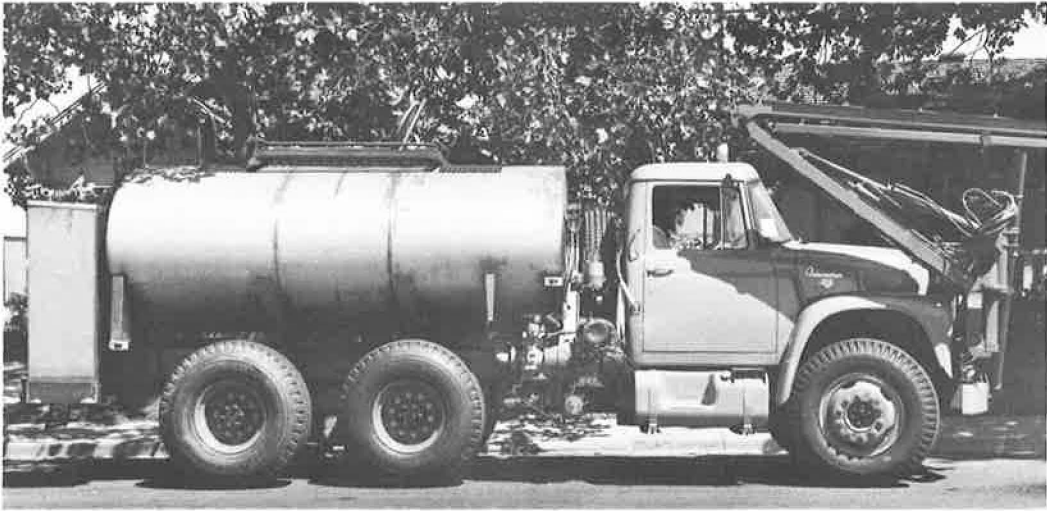
Figure 1. Overall unit as tested, showing main and proportioning pump mounted near cab.
