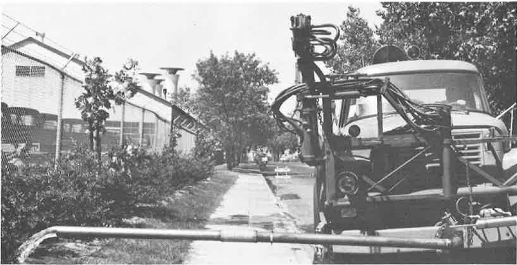
Figure 2. Front view with spray boom folded in travel position and unit being used for irrigating roadside ornamentals (water pipe air actuated for quick lifting to clear signs, etc.).
