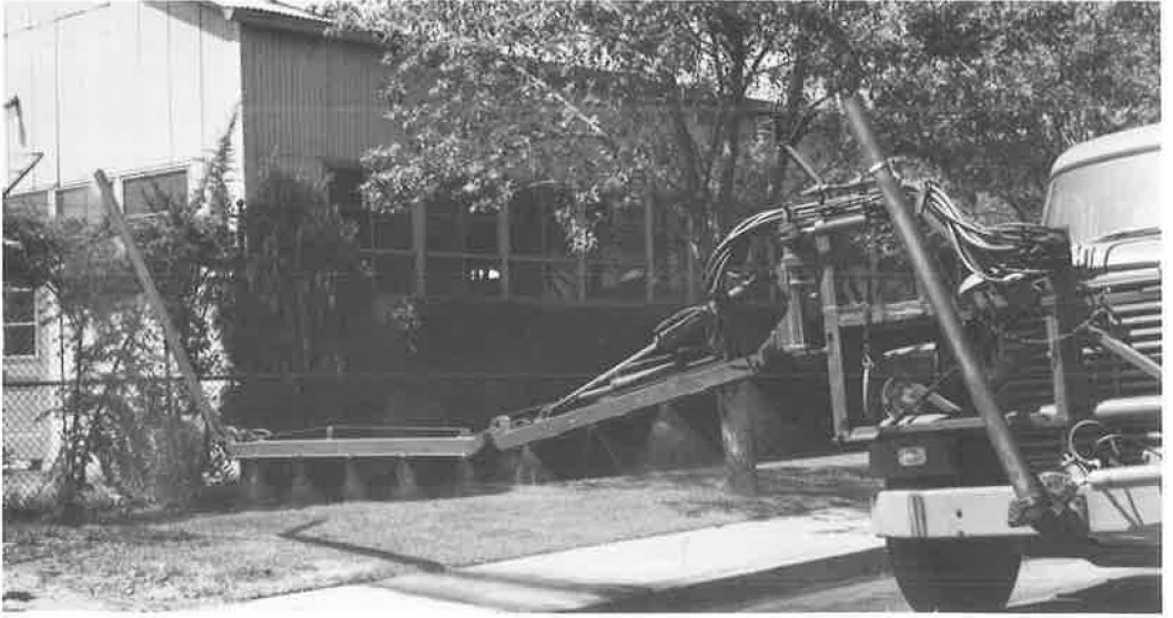
Figure 3. Spray boom in operation with irrigation pipe in travel position.
