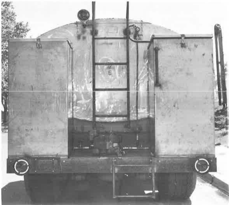
Figure 4. Rear view showing two chemical tanks and agitating engine with drive belts beneath platform and retractable rear step.
