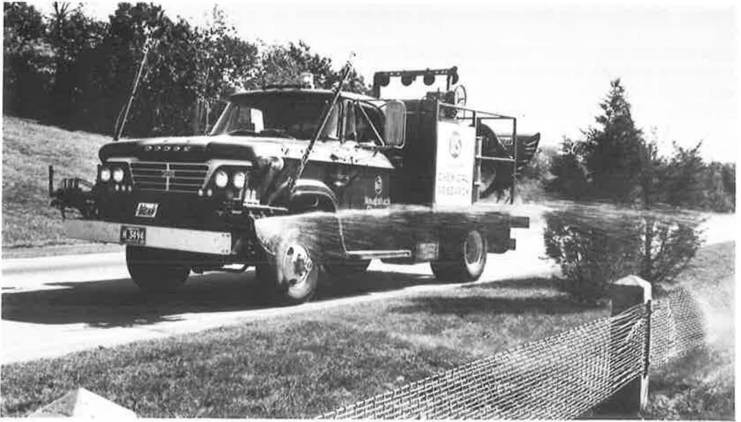
Figure 2. Maleic hydrazide spray application for grass inhibition.
